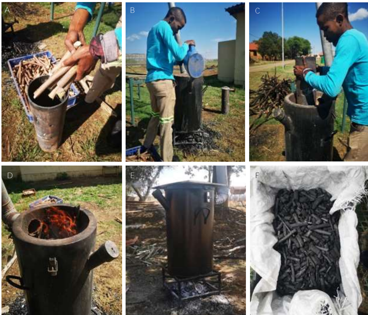
Figure 2. Biochar production steps . A) cooker compartment being loaded with feedstocks, B) boiler being filled with water, C) cooker compartment placed in the middle of the stove, D and E) a fire was prepared outside the cooker compartment and a lid placed on the kiln stove, F) biochar removed from the cooker (after cooling if with a bit of water and air-dried).
