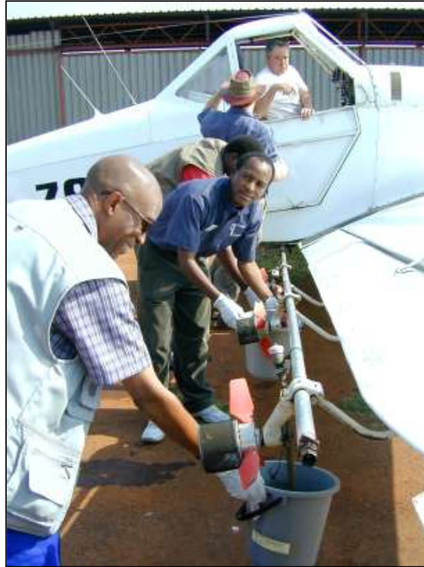
Fig.5. ICOSAMP delegates learning how to calibrate atomizer nozzles on the aircraft.
