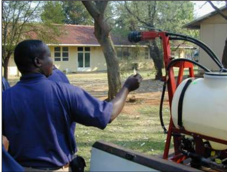
Fig.3. Collection of spray droplets on a magnesium oxide slide from a vehicle mounted sprayer
