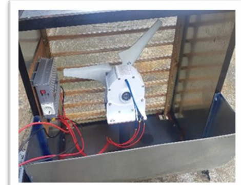
Figure 2: Small wind turbine prototype showing (a) the front side of the wind turbine with a louvre mechanism, (b) the open louvre mechanism, and (c) the inside of the small wind turbine prototype
