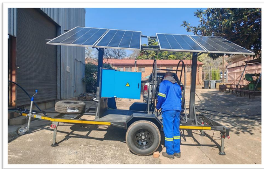
A mobile solar power trailer that can be towed around the farm for water abstraction
