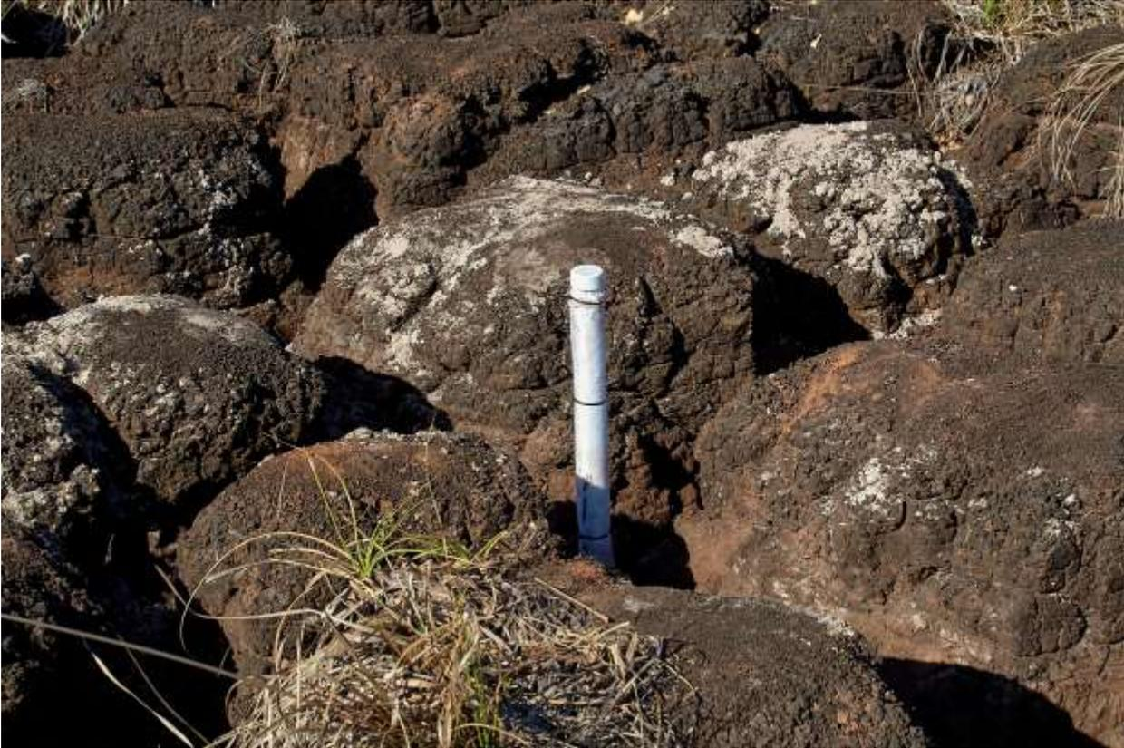
Figure 1: Vazi peatland with monitoring well installed to measure the water level.
