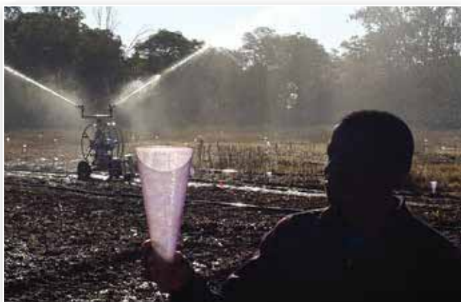
Evaluation of travelling irrigators to determine its performance.
