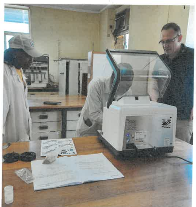
Figure 3: Sample preparation for spectral analysis using a Retsch MM400 mixer ball miller.
