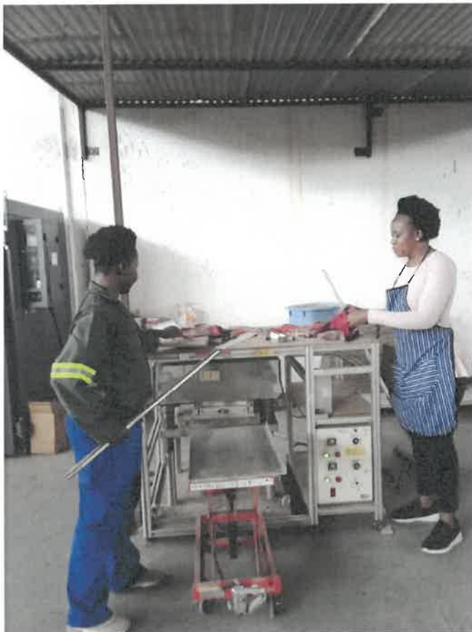
Loading the form into the heat compressor
