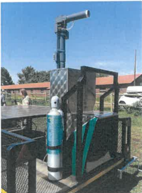
The mobile GreenFeeds system, which operates with sun panels and a battery, is used in the dairy department. (Photograph: supplied by the ARC).
