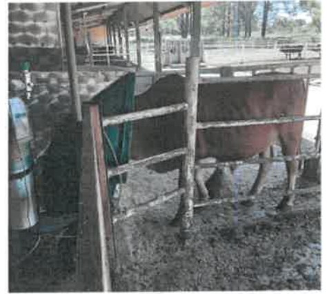
The GreenFeeds system collects methane gas when an animal feeds and then releases gas. (Photograph: supplied by the ARC)
